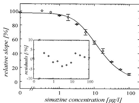
Fig. 10. Titration curve of antibody KIF4 by simazine and fit of the free binding site model. The residuals of the fit are shown in the inset.
