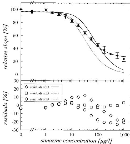
Fig. 11. Titration of antibody K4G2 by simazine and fitting of simple model (—), a model taking an offset into account (- - -) and a fit of the beginning (0–10  $\mu\text{g/l}$ ) of the titration curve ( $\cdot\cdot\cdot$ ). The residuals of all three fits are shown in the bottom diagram.
