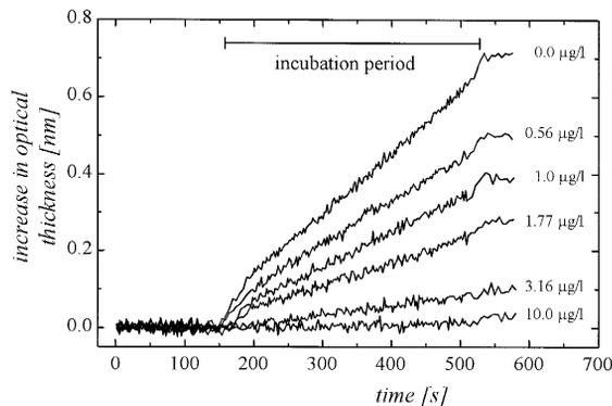
Fig. 8. Binding curves for 0.5  $\mu\text{g}/\text{ml}$  K1F4 at various concentrations of terbuthylazine.
