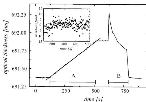
Fig. 6. Typical test cycle for the determination of free antibodies binding sites. Injection of  $0.75 \mu\text{g/ml}$  mab K4G2 without any analyte (section A) and regeneration by incubation of  $2 \text{ mg/ml}$  pepsin pH 2 (section B). The inset shows the residuals of a linear regression of the binding curve.
