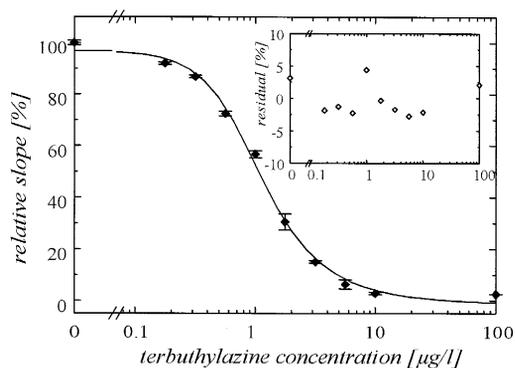
Fig. 9. Titration curve of terbuthylazine with antibody KIF4, 1  $\mu\text{g}/\text{ml}$ , and fitting by the model described above for IgG (line). The residuals of the fit are shown in the inset.
