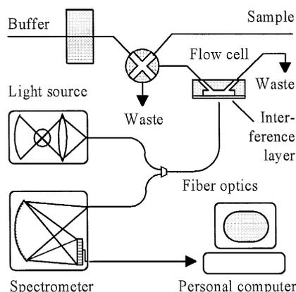
Fig. 4. Schematic set-up for monitoring of affinity interactions by RIFS.
