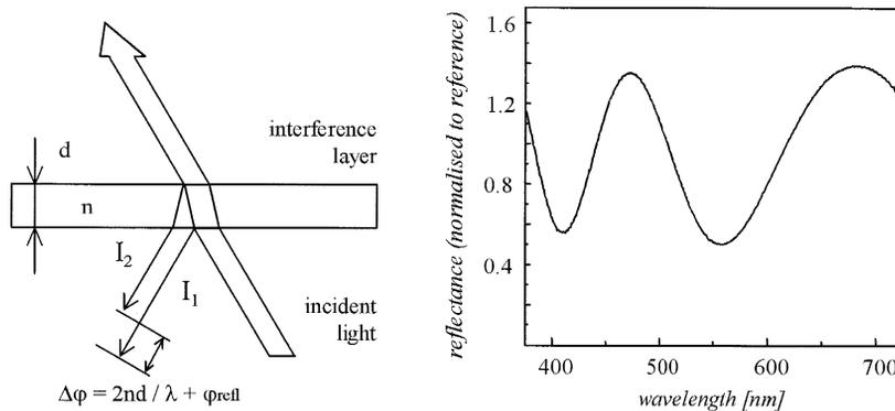
Fig. 3. Detection principle of RIfS: The increase in thickness of a thin layer is detected as a change in the pattern of the interference spectrum.
