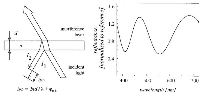
**FIG. 2.** Principle of the detection of affinity interactions by RIFS ( $n$  and  $d$  are the refractive index and the thickness of the layer,  $I_1$  and  $I_2$  are the intensities of the reflected light beams,  $\Delta\phi$  is the difference in the optical path length of the two beams, and  $\phi_{\text{ref}}$  is the phase shift upon reflection).
