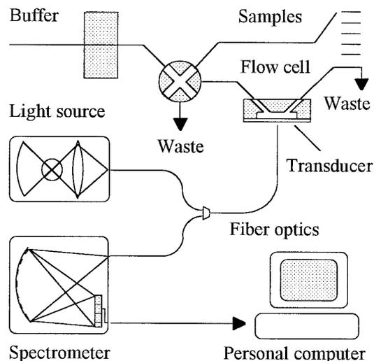
**FIG. 3.** Experimental setup used for monitoring binding events.
