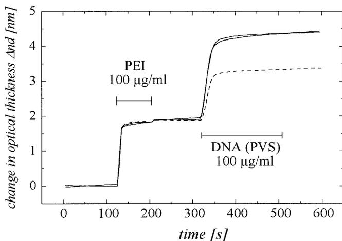
FIG. 4. Immobilization of DNA (—) and PVS (· · ·) after pretreatment of the surface with PEI.
