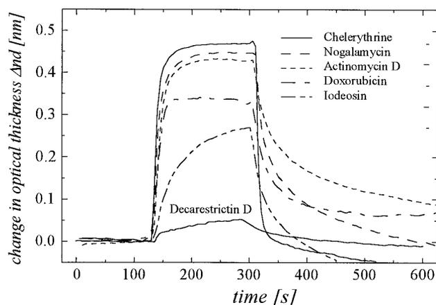
**FIG. 5.** Sensor response during incubation of various intercalators and other compounds at a concentration of 10  $\mu\text{g/ml}$ .
