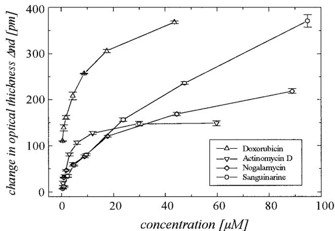
**FIG. 7.** Adsorption isotherms for intercalator binding to immobilized DNA.
