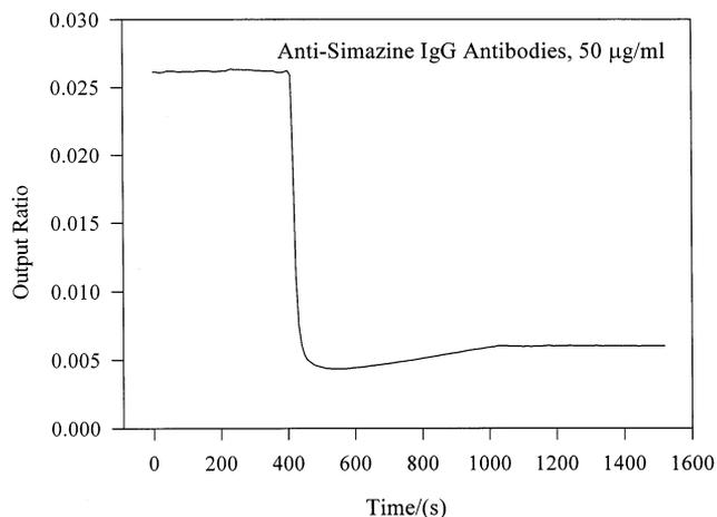
Fig. 5. Response to high anti-simazine IgG antibody loading of the sensor surface.
