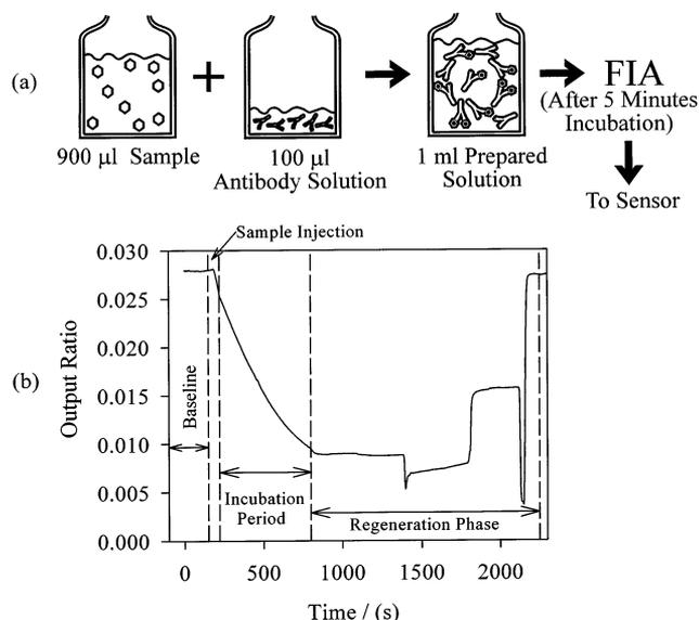
Fig. 4. IOSPR immunoprobe test-cycle: (a) Sample preparation; and (b) Sensor output ratio during the test-cycle.
