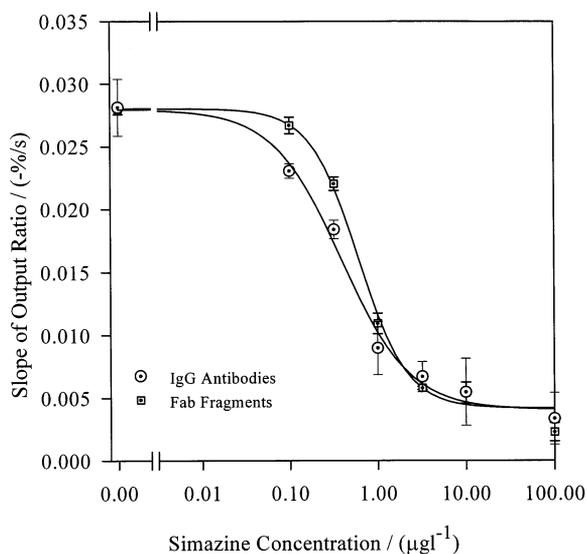
Fig. 8. IOSPR immunoprobe averaged triplicate anti-simazine IgG antibody calibration curve and averaged duplicate anti-simazine Fab fragment calibration curve.
