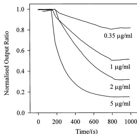
Fig. 6. System characterisation for reducing concentrations of anti-simazine IgG antibodies. A linear binding regime has been achieved by an antibody concentration of 0.35  $\mu\text{g/ml}$ .
