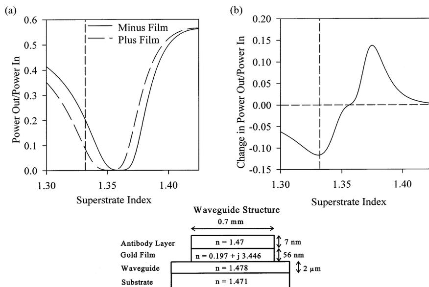
Fig. 2. Theoretical operating curves for a Pyrex IOSPR sensor at 633 nm incorporating a diagram of the waveguide structure modelled. The refractive index of water is shown as a dashed vertical line on each graph.
