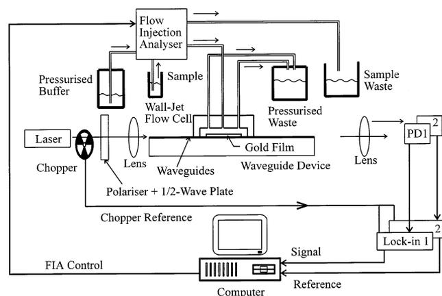
Fig. 3. Experimental set-up of the computer controlled FIA IOSPR immunoprobe system.
