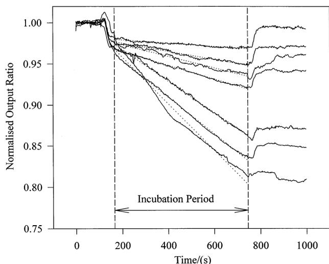
Fig. 7. Real-time immunoprobe response for several simazine concentrations over the range of 0–100  $\mu\text{g/l}$ .
