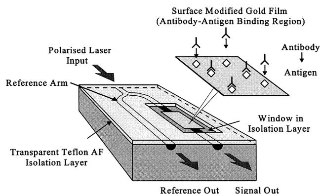
Fig. 1. Schematic diagram of the integrated optical SPR immunoprobe showing the binding of antibodies to the surface modified gold film.
